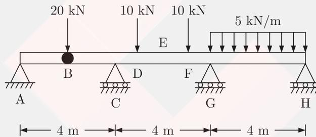
$$\begin{aligned} AB &= BC = 2 \text{ m} \\ CD &= DE = EF = FG = 1 \text{ m} \\ GH &= 4 \text{ m} \end{aligned}$$
