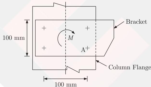
The shear force induced in the rivet A is
