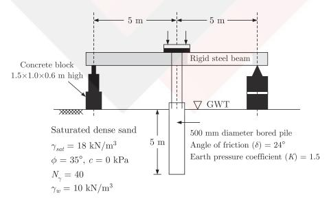
The maximum pressure that can be applied with a factor of safety of 3 through the concrete block, ensuring no bearing capacity failure in soil using Terzaghi's bearing capacity equation without considering the shape factor, depth factor and inclination factor is
