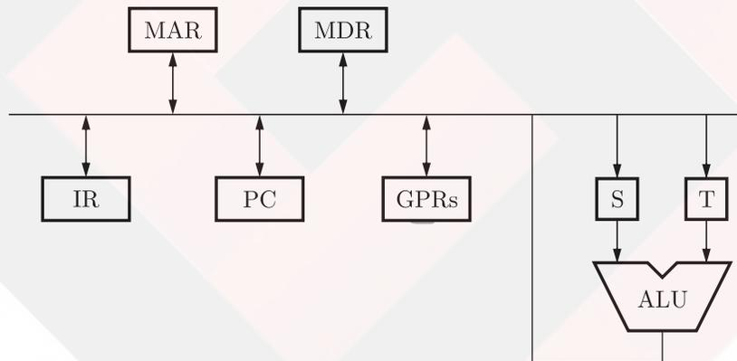
The, ALU, the bus and all the registers in the data path are of identical size. All operations including incrementation of the PC and the GPRs are to be carried out in the ALU. Two clock cycle are needed for memory read operation-the first one for loading data from the memory but into the MDR.
