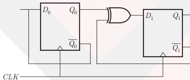
The flip-flops are positive edge triggered *DFFs*. Each state is designated as a two bit string  $Q_0, Q_1$ . Let the initial state be 00. The state transition sequence is
